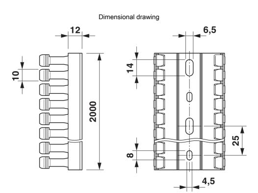
Base perforation according to DIN EN 50085
